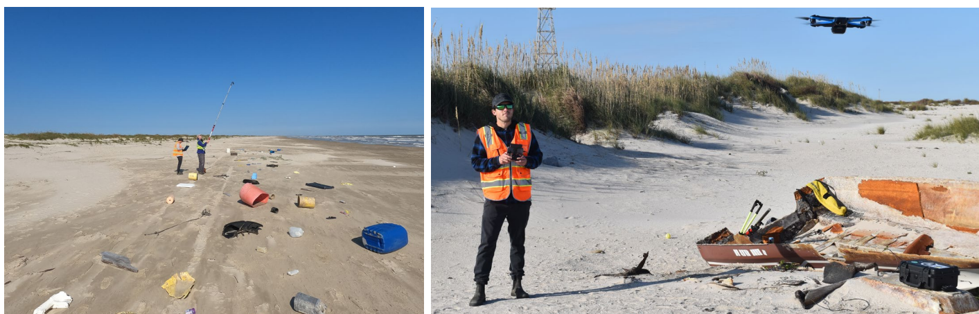
Image 12 (left): Researchers test a polarimetric camera on a pole-mounted platform to test marine debris detecting software. Image 13(right): UAS operator flies a UAS over marine debris to test detection (right). Photo: Kyle Herrera/OSU
