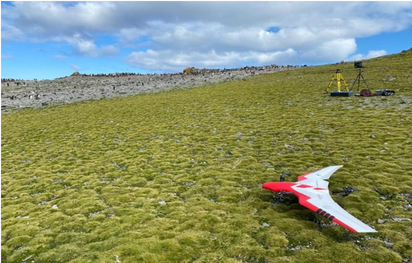
Image 9: Preparing the FireFly 6 Pro UAS for mapping missions over Adelie and Gentoo penguin colonies. Photo: SWFSC/NOAA
